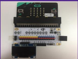
Put the micro:bit into the Breakout Board and put the OLED onto any of the 4 holes seen at the bottom of the Breakout Board.
